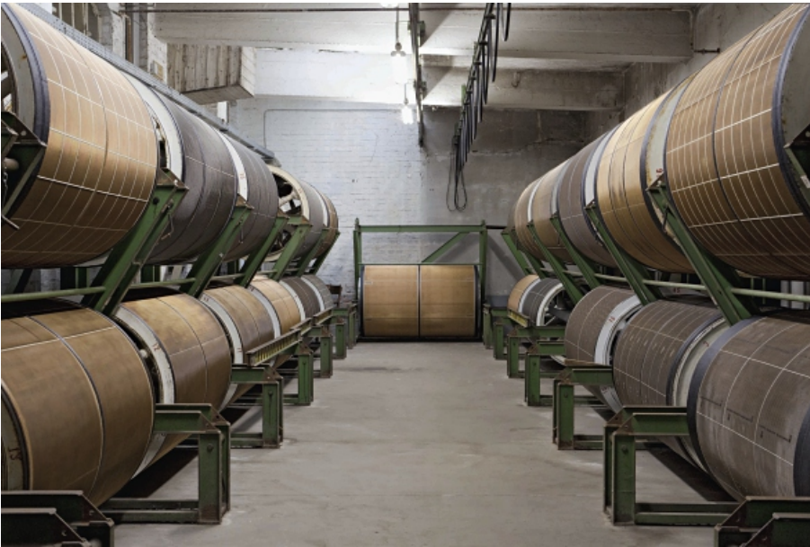
Cylinder molds for making mold-made papers. Cotton fibers and cellulose are the paper raw materials.
